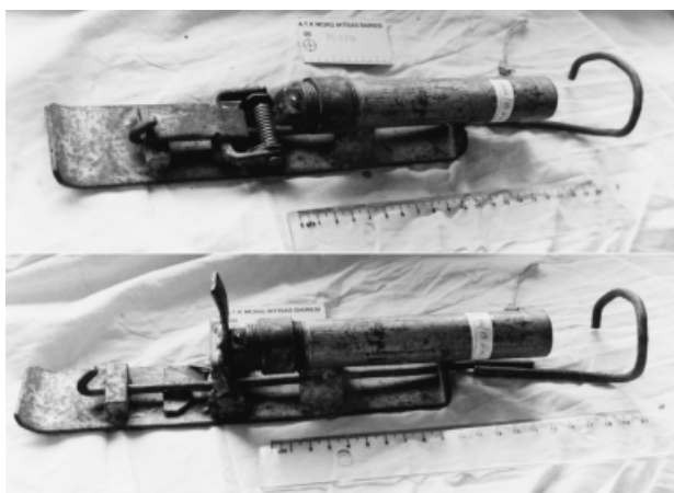
FIG. 2—A mole gun with its trigger mechanism. The upper one is ready to fire, and the bottom one is fired.
